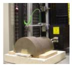
• Fixed inductor under the workpiece.
