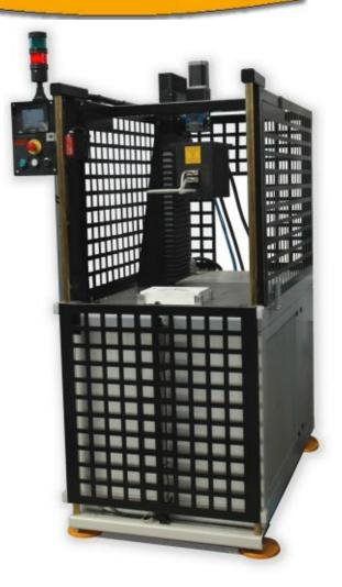
Each machine is assembled on a steel **mainframe**, where there are the electric cabinet and the working bench, complete of adequate metallic safety barriers.
