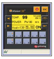
The electric cabinet contains all the electrical components, the power generator, the cooler and the **control panel** complete of a PLC with a display for the set up and the control of the working parameters.
