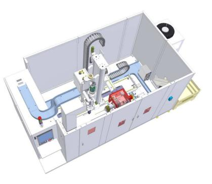
make single pass welding of thickness from 1 to 2,5 mm and a deposition rate till 2 kg/h respecting severe metallurgical parameters.
